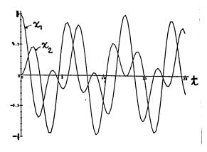
Plot obtained using the Maple command with (plots): implicit plot ({x = 0.5 \* co(t)  $+0.5*\cos(\text{sqxt}(3)*t), \chi =$ 0.5\*co(t) - 0.5\*co(agrt(3)\*t)t=0..20, x=-2..2,numpoints =6000);
