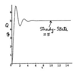
$2Q''+4Q'+20Q=10(1-\bar{e}^{t}), Q(0)=Q'(0)=0$ The maple doolie solution is very massy, so let's solve by hand.  $Q_{R}=e^{-t}(C_{1}c_{1}3t+C_{2}si_{1}3t)$  and seek  $Q_{1}=A+Be^{-t}$ . This gives A=1/2,B=-5/9As  $Q(t)=\frac{1}{2}-\frac{5}{9}e^{t}+e^{t}(C_{1}c_{1}3t+C_{2}si_{1}3t)$  Q(0)=0 and Q'(0)=0 give  $C_{1}=1/18$  and  $C_{2}=-1/6$ , so  $Q(t)=\frac{1}{2}-\frac{5}{9}e^{t}+e^{t}(\frac{c_{1}3t}{18}-\frac{si_{1}3t}{6})$ Steady-state solution is  $Q(t)\to 1/2$
