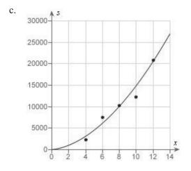
11. Students in a lab measured the breaking strength S (in pounds) of wood 2 inches thick, x inches high, and 12 inches long. The results are shown in the table below. Use the model  $S = 180.89x^2 - 205.79x + 284$  to approximate the breaking strength when x = 2. Round your answer to two decimal places.
