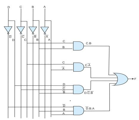
38. Consider the following circuit that takes a 4-bit binary input and encodes it. Construct a truth table for the 16 inputs 0000 to 1111 and examine the output code. What is the characteristic feature of this code?
