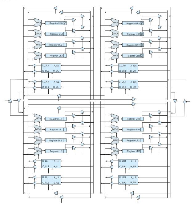
Essentially, this replicates a basic register and ALU circuit four times. In each quadrant data can be moved from registers to the ALU and back to registers. Note that the four buses and two ALUs permit parallel operations (two ALU operations at a time).
