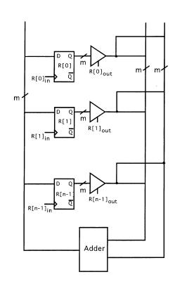
2.29 Design data path logic that will allow any two of the following register transfers that do not have the same destination to be done in one step. (§2.5)
