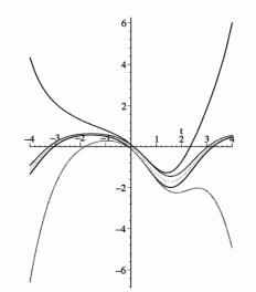
The three middle curves are the solutions to the differential equation corresponding to the initial conditions x(0) = -.1, 0.1, and the outside curves are the graphs of  $e_L$  and  $e_H$ . Note how the solutions of the differential equation remain inside the graphs of  $e_L$  and  $e_H$ .
