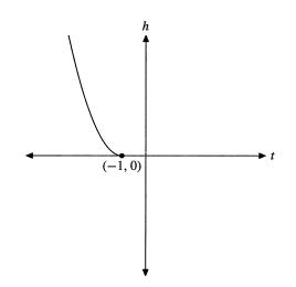
(b) Let A represent the cross area of the drum and h the height of the water in the drum. Then Δh represents the change in height and AΔh the volume of water that has left the drum. A particle of water leaving the drain at speed v travels a distance vΔt in a time Δt. Because a is the cross section of the drain, the volume of water leaving the drain in time Δt is avΔt. Because the water leaving the drum in time Δt must exit the drain,
