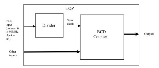
Synthesize the top module (which includes the divider and the 1-digit bcd counter) and use the following pin assignments. Download the design onto the board and make sure it works as expected.
