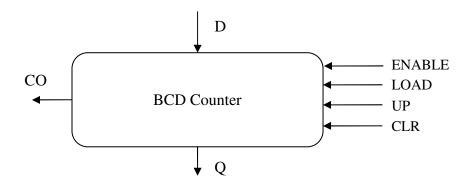
If the LOAD = ENABLE = 1, the data input D is loaded into the counter.
