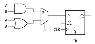
Unlike *Clr*, the output from the mux is only read on falling clock edges; therefore, adding *C* to the sensitivity list is not required for proper operation of the circuit.
