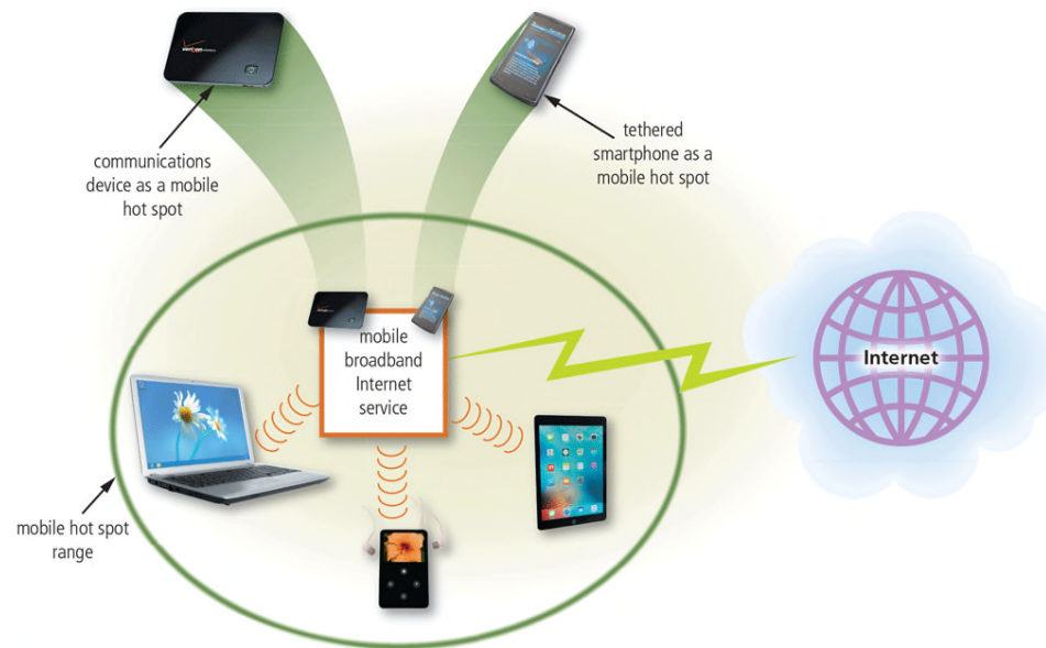
Figure 2-3 You can create a mobile hot spot using a communications device or by tethering a smartphone. Courtesy of Verizon Wireless; figarro / Can Stock Photo; iStockphoto.com / Mlenny; amfoto / Shutterstock.com; Alex Staroseitsev / Shutterstock.com; Source: Microsoft
