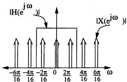
From the sketch, we observe that the LTI system is a lowpass filter which removes all but three of the frequency impulses. To these, it multiplies a phase factor  $e^{-j3\omega}$ .
