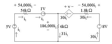
[a] To find  $i_1$ , write a KVL equation around the left-hand loop, summing voltages in a clockwise direction starting below the 5V source:
