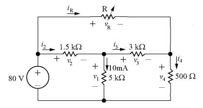
Ohms' law for 5 k $\Omega$  resistor:  $v_1 = (0.01)(5000) = 50 \text{ V}$
