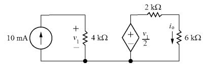
$$v_1 = (4000)(0.01) = 40 \,\text{V}$$
