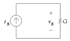
[a] Note from the circuit that the current through the conductance G is  $i_g$ , flowing from top to bottom, because the current source and the
