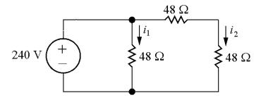
Write a KVL equation for the left and right loops:
