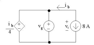
[a] Note that the current  $i_b$  is in the same circuit branch as the 8 A current source; however,  $i_b$  is defined in the opposite direction of the current source. Therefore,
