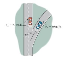
At the instant shown, cars A and B travel at speeds of 70 mi/h and 50 mi/h, respectively. If B is decreasing its speed at 1400 mi/h<sup>2</sup> while A is increasing its speed at 800 mi/h<sup>2</sup>, determine the acceleration of B with respect to A. Car B moves along a curve having a radius of curvature of 0.7 mi.
