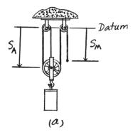
If the rope is drawn toward the motor M at a speed of  $v_M = (5t^{3/2})$  m/s, where t is in seconds, determine the speed of cylinder A when t = 1 s.
