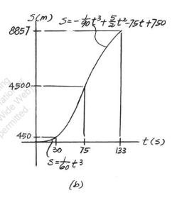
The snowmobile moves along a straight course according to the v-t graph. Construct the s-t and a-t graphs for the same 50-s time interval. When t = 0, s = 0.
