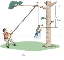
The man pulls the boy up to the tree limb C by walking backward. If he starts from rest when  $x_A = 0$  and moves backward with a constant acceleration  $a_A = 0.2 \text{ m/s}^2$ , determine the speed of the boy at the instant  $y_B = 4 \text{ m}$ . Neglect the size of the limb. When  $x_A = 0$ ,  $y_B = 8 \text{ m}$ , so that A and B are coincident, i.e., the rope is 16 m long.
