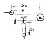
If block B is moving down with a velocity  $v_B$  and has an acceleration  $a_B$ , determine the velocity and acceleration of block A in terms of the parameters shown.
