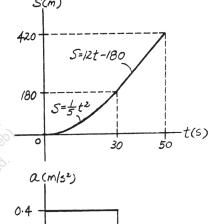
$a = \frac{dv}{dt}$ . For time interval  $0 \text{ s} \le t < 30 \text{ s}$  and  $30 \text{ s} < t \le 50 \text{ s}$ ,  $a = \frac{dv}{dt} = \frac{2}{5}$
