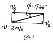
The box slides down the helical ramp which is defined by r = 0.5 m,  $\theta = (0.5t^3) \text{ rad}$ , and  $z = (2 - 0.2t^2) \text{ m}$ , where t is in seconds. Determine the magnitudes of the velocity and acceleration of the box at the instant  $\theta = 2\pi \text{ rad}$ .
