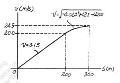
The v-s graph for the car is given for the first 500 ft of its motion. Construct the a-s graph for  $0 \le s \le 500$  ft. How long does it take to travel the 500-ft distance? The car starts at s = 0 when t = 0.
