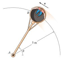
Car B turns such that its speed is increased by  $(a_t)_B = (0.5e^t) \text{ m/s}^2$ , where t is in seconds. If the car starts from rest when  $\theta = 0^\circ$ , determine the magnitudes of its velocity and acceleration when t = 2 s. Neglect the size of the car.
