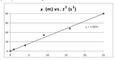
The plot yields a best-fit line with slope  $a/2 = 1.6 \text{ m/s}^2$ . Thus, the acceleration of the car is approximately 3.2 m/s<sup>2</sup>. ASSESS This is about 0.3g. For Formula One race, the initial acceleration is typically around 1.5g.
