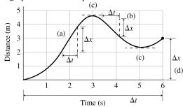
EVALUATE (a) The largest instantaneous velocity in the positive-x direction occurs at approximately t = 2 s and is approximately  $v = dx/dt \approx \Delta x/\Delta t = (1.8 \text{ m})/(0.6 \text{ s}) = 3 \text{ m/s}.$
