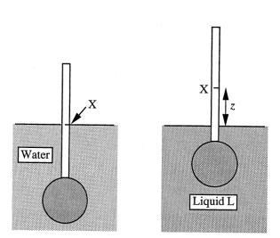
Since the same weight (that of the hydrometer) is supported by the displaced liquid in Both Cases:
