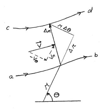
Mass flow between streamlines =  $\Delta \bar{\psi}$
