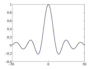
9.  $x_9(t)$  is the product of a sinusoidal signal with frequency 2 and an expanded rectangular pulse.
