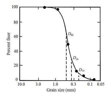
b. From the graph,  $D_{60} = 0.48 \text{ mm}$ ,  $D_{30} = 0.33 \text{ mm}$ ,  $D_{10} = 0.23 \text{ mm}$
