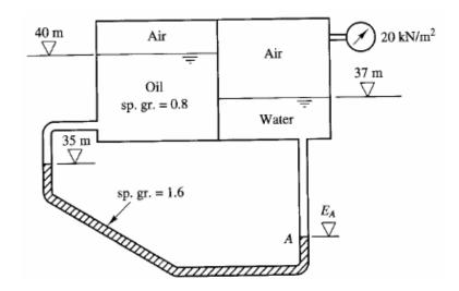
Ans. Using the "swim through" technique, start at the right tank where pressure is known and "swim through" the tanks and pipes, adding pressure when "swimming" down and subtracting when "swimming" up until you reach the known pressure in the left tank. Solve for the variable elevation  $(E_A)$  in the resulting equation.
