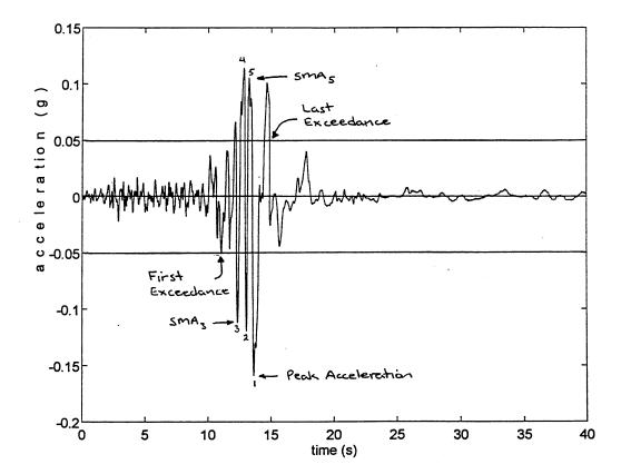
3.2 Integrate the time history of acceleration to produce time histories of velocity and displacement. Plot the time histories of velocity and displacement and determine the peak velocity and peak displacement.
