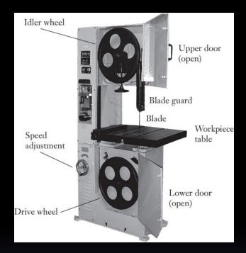
A variable-speed motor enables the operator to adjust the blade's speed depending on the type and thickness of the material being cut.
