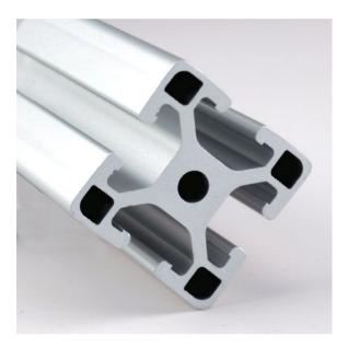
This was most likely manufactured using an extrusion process because of the material and constant cross section geometry of the member. Shorter pieces could be die cast, although longer pieces are most certainly extruded. Machining could be another option for very small pieces, although machining would be much more time consuming for a part like this.
