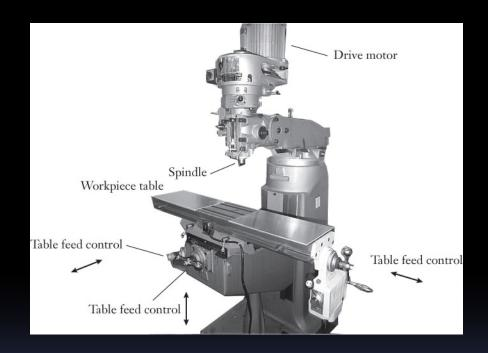
The workpiece is held by a vise on an adjustable table so that the part can be accurately moved in three directions.
