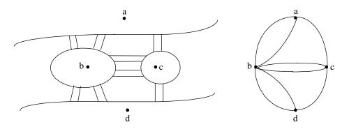
If we want a walk that returns to its starting point, all the vertices in the corresponding multigraph must be even. Since a new bridge/edge changes the parity of two vertices, at least two new bridges/edges will be needed. For example, here is one such "enhancement":
