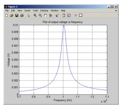
(b) The resonant frequency of this circuit is about 1.007 MHz. If the frequency is changed to 1.1 MHz, the output voltage will be 1.75 mV instead of the 10 mV at the resonant frequency. This receiver is not very selective—real radios do *much* better.
