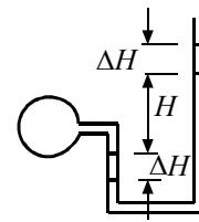
2.40  $p + 9810 \times 0.05 + 1.59 \times 9810 \times 0.07 - 0.8 \times 9810 \times 0.1 = 13.6 \times 9810 \times 0.05.$
