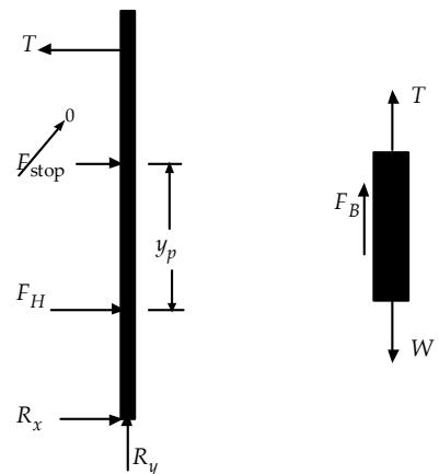
$$F_H = \gamma \bar{h} A = (9.81 \text{ kN/m}^3)(1.5 \text{ m} \times 6 \text{ m}^2) = 88.29 \text{ kN}$$
