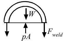
2.77 A free-body diagram of the gate and water is shown.
