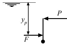
2.56  $F = \gamma \bar{h} A = 9810 \times 6 \times 20 = 1.777 \times 10^6 \text{ N, or } 1177 \text{ kN.}$
