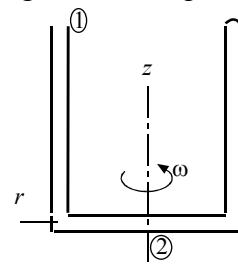
d)  $0 = \frac{1}{2} \times 1.94 \omega^2 \left( -\frac{11.25^2}{12^2} \right) - 62.4 \left( -\frac{15}{12} \right)$ .  $\therefore \omega = 9.57 \text{ rad/s}$
