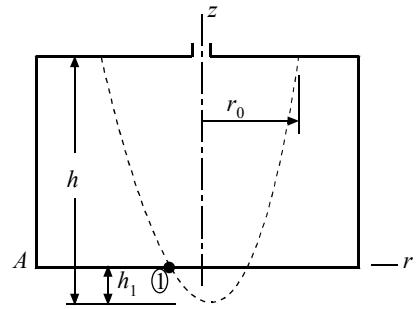
Also,  $h - h_1 = 0.8$ .  $1.6h - 0.64 = 0.7339$ .  $\therefore h = 0.859 \text{ m}$ ,  $r_1 = 0.108 \text{ m}$ .
