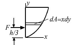
$$W = 9810 \int_0^2 2x dy = 9810 \int_0^2 2 \frac{y^{1/2}}{\sqrt{2}} dy = \frac{2 \times 9810}{\sqrt{2}} \frac{2^{3/2}}{3/2} = 26\ 160 \text{ N.}$$
