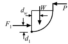
Note: This calculation is simpler than that of Example 2.7. Actually, We could have moved the horizontal force  $F_H$  and a vertical force  $F_V$  (equal to  $W$ ) simultaneously to the center of the circle and then  $2.5P = 2F_H = 2F_1$ . This was outlined at the end of Example 2.7.
