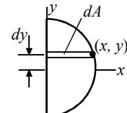
c)  $F = 9810 \times (4 + 4/3) \times 6 = 313\,900 \text{ N or } \underline{313.9 \text{ kN.}}$
