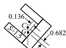
$$\text{b) } \bar{y} = \frac{4 \times 2 + 2 \times \frac{1}{2} + 2 \times 3.5}{4 + 2 + 2} = 2. \quad \bar{x} = \frac{4 \times \frac{1}{2} + 2 \times 2 + 2 \times 2}{4 + 2 + 2} = 1.25$$
