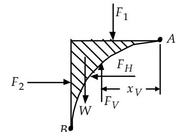
The line of action of  $F_H$  is the same as that of  $F_2$ . Its distance from the surface is
