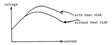
For low currents Ohm's law applies and the current is directly proportional to the applied voltage in both cases. The thermistor temperature is that of its surroundings. The system with a heat sink can reach higher current levels and still remain in a linear portion of the v-i curve since the heat sink keeps the thermistor at approximately the ambient temperature. Eventually the thermistor–heat sink combination will self heat and a negative-resistance relationship will result.
