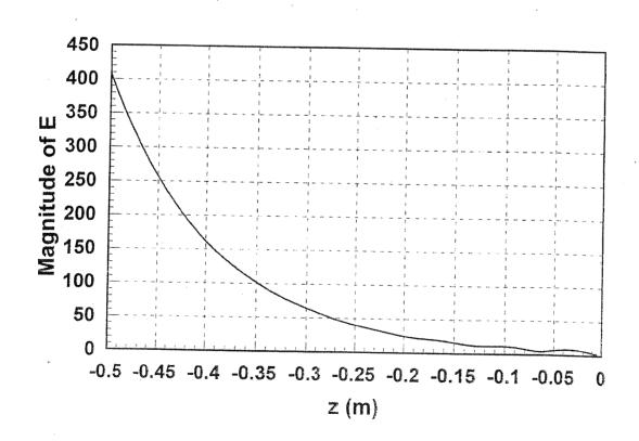
(1.10) The total loss through the sheet is the product of the transmission losses at the air-copper and copper-air interfaces, and the exponential loss through the sheet.
