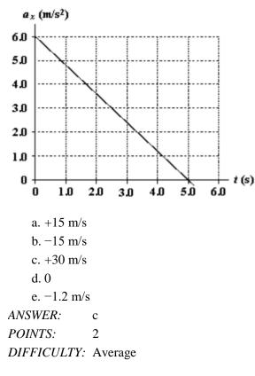
10. At t = 0, a particle is located at x = 25 m and has a velocity of 15 m/s in the positive x direction. The acceleration of the particle varies with time as shown in the diagram. What is the position of the particle at t = 5.0 s?
