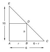
We write a proportion involving the lengths of the sides of the similar triangles BCD and ACE. Then we solve it for h.
