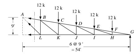
Using the method of sections and considering the force in member AL to act at L,
