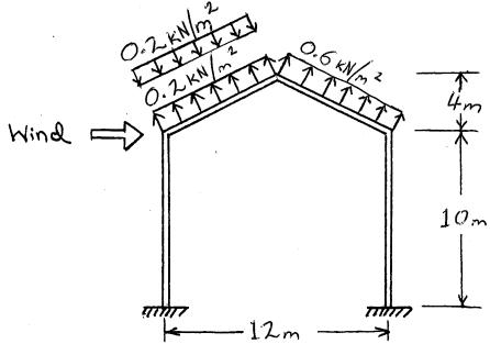
[2.11] V = 40m/s, E = 1.15, 3g = 274.32m,  $\alpha = 9.5$ From the solution of Problem 2.10:  $9h = 1.17 \, \text{kN/m}^2$  and G = 0.85
