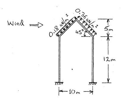
[2.9]  $V = 40 \text{ m/8}, h = 12 + \frac{5}{2} = 14.5 \text{ m}$   $I = 1.15, 8_{9} = 366 \text{ m}, \alpha = 7.0, K_{8t} = 1$ and  $K_{d} = 1$   $K_{h} = 2.01 \left( \frac{14.5}{366} \right)^{2} = 0.8$   $Q_{h} = 0.613(0.8)(1)(1)(40^{2}(1.15) = 902.34 \text{ N/m}^{2})$  A = 0.85Roof slope:  $\Theta = \tan^{-1}(5/6) = 39.8^{\circ}$   $\frac{h}{L} = \frac{14.5}{12} = 1.21$  Cp = -0.1 and 0.25 for windward side
