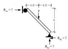
$\sum M_{B} = 0 \qquad \sum F_{X} = 0$   $(P * L/2) - (R_{Ax} * h) = 0 \qquad R_{Ax} + R_{Bx} = 0$   $(R_{Ax} * h) = PL/2 \qquad R_{Bx} = -R_{Ax}$   $R_{Ax} = PL/2h \rightarrow \qquad R_{Bx} = PL/2h \leftarrow$
