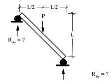
$R_{By} * L = PL/2 \qquad R_{Ay} = P - R_{By}$  $R_{By} = P/2 \uparrow \qquad R_{Ay} = P - P/2$  $R_{Ay} = P/2 \uparrow$  $R_{Ay} = P/2 \uparrow$
