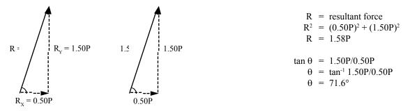
Question 2.3: The following three forces act concurrently through a point: a force P acting to the right at  $\theta_x = 30^\circ$  to the horizontal, a force P acting to the right at  $\theta_x = 45^\circ$  to the horizontal, and a force P acting to the right at  $\theta_x = 60^\circ$  to the horizontal. Find the single resultant force that is equivalent to this three-force system.
