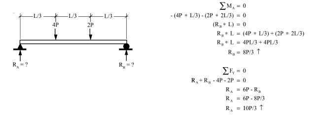
Question 2.10: Determine the reactions for the structure shown in Figure 2.59(Q10).
