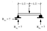
$$\begin{split} \sum M_{A} &= 0 & \sum F_{Y} &= 0 \\ (R_{By} * L) - (P * L/2) &= 0 & R_{Ay} + R_{By} - P &= 0 \\ R_{By} * L &= PL/2 & R_{Ay} = P - R_{By} \\ R_{By} &= P/2 \uparrow & R_{Ay} &= P - P/2 \\ R_{Ay} &= P/2 \uparrow & \\ \sum F_{X} &= 0 \\ R_{Ax} &= 0 \end{split}$$
