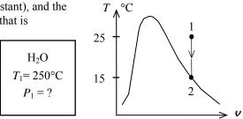
**3-61** Heat is supplied to a piston-cylinder device that contains water at a specified state. The volume of the tank, the final temperature and pressure, and the internal energy change of water are to be determined.
