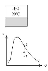
**3-53** A piston-cylinder device contains a saturated liquid-vapor mixture of water at 800 kPa pressure. The mixture is heated at constant pressure until the temperature rises to 200°C. The initial temperature, the total mass of water, the final volume are to be determined, and the P-v diagram is to be drawn.
