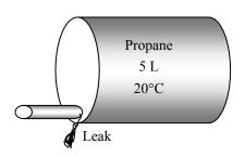
**3-132** An isobutane tank contains 5 L of liquid isobutane at the ambient temperature. Now a leak develops at the top of the tank and isobutane starts to leak out. The temperature of isobutane when the pressure drops to 1 atm and the amount of heat transferred to the tank by the time the entire isobutane in the tank is vaporized are to be determined.
