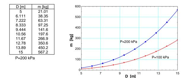
3-78 Two rigid tanks connected by a valve to each other contain air at specified conditions. The volume of the second tank and the final equilibrium pressure when the valve is opened are to be determined.
