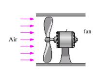
**2-49** The fan of a central heating system circulates air through the ducts. For a specified pressure rise, the highest possible average flow velocity is to be determined.
