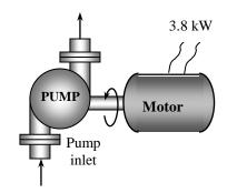
**Discussion** The conservation of energy principle requires the energy to be conserved as it is converted from one form to another, and it does not allow any energy to be created or destroyed during a process. In reality, the volume flow rate will be less because of the losses associated with the conversion of electrical-to-mechanical shaft and mechanical shaft-to-flow energy.
