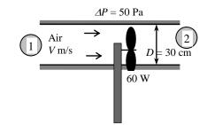
**Discussion** The conservation of energy principle requires the energy to be conserved as it is converted from one form to another, and it does not allow any energy to be created or destroyed during a process. In reality, the velocity will be less because of the losses associated with the conversion of electrical-to-mechanical shaft and mechanical shaft-to-flow energy.
